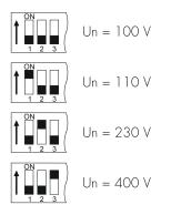
Figure 4.3: Adjustment of rated voltage
