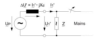
Figure 3.3: Equivalent circuit at mains failure
