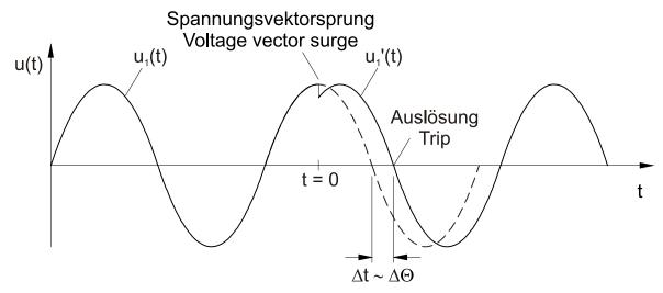
Figure 3.5: Voltage vector shift
