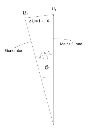
Figure 3.2: Voltage vectors at mains parallel operation
