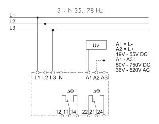
Figure 2.2: Connection three--wire system  $\Delta$
