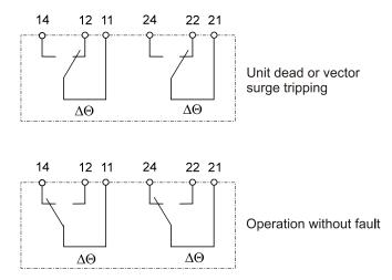
Figure 2.4: Contact positions of the output relays
