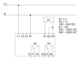
Figure 2.1: Connection two-wire system
