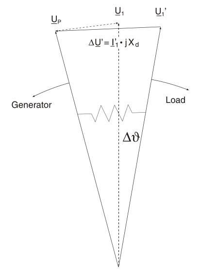
Figure 3.4: Voltage vectors at mains failure
