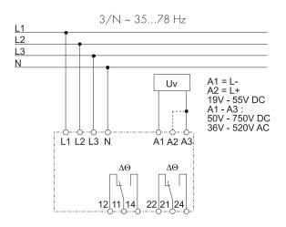
Figure 2.3: Connection four-wire system Y/Δ
